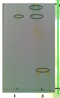
Fig. 3b. Detection system (vanillin – acetic acid)
